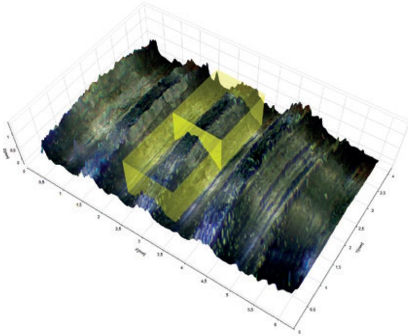
With the 3D module in InSight, it is possible to display a 3D model of the specimen under observation.
