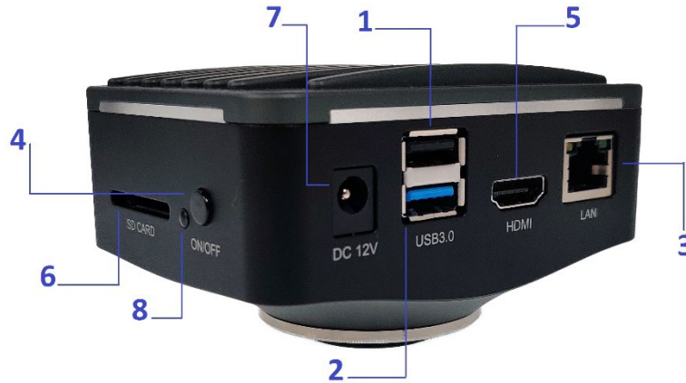
Figure 2-1 Available Ports on the Back Panel of the Camera
